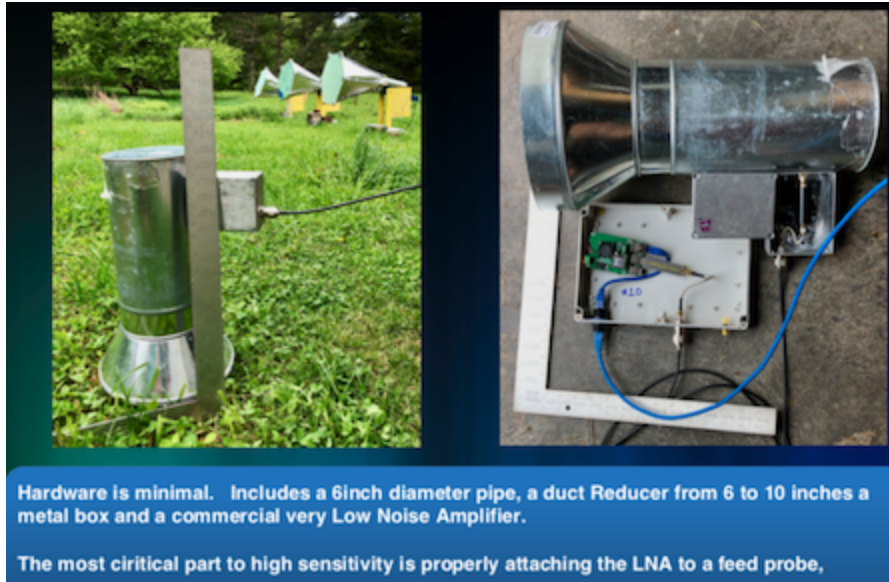
Figure 2: Left is the horn. At right is the side view of the horn and the computer box containing the SDR and the Raspberry Pi 4 computer. The Pi is powered by the blue ethernet cable, which also connects the Pi to the computer network. The Pi is in a weatherproof box.
