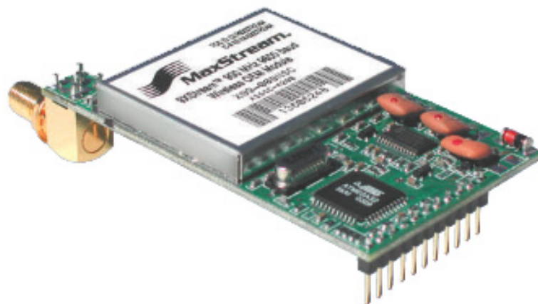
Figure A.4: Photo of the XStream 900MHz radio modem module.
